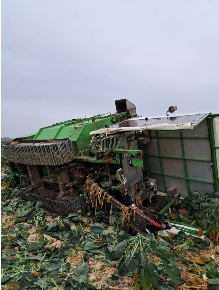
Appendix 3: T.H. Clements harvesting equipment toppled in unstable soils
